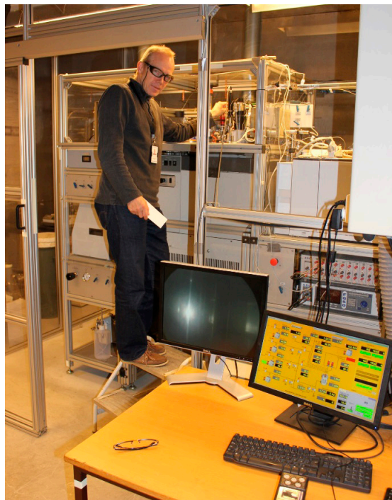
Dr Jacob Stang working on the vapour-liquid equilibrium setup. Photo: SINTEF/Sigurd W. Løvseth.
